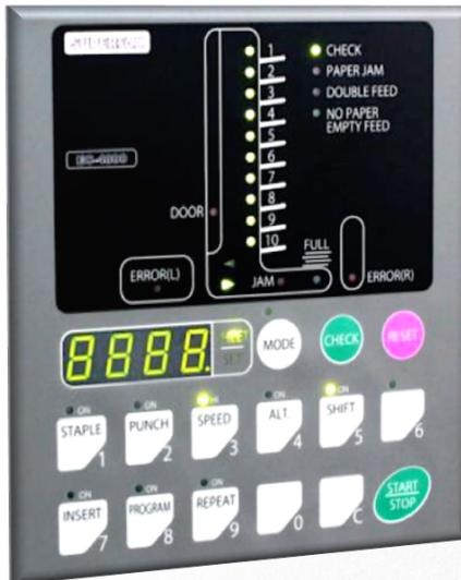
*All the functions are effectively dis-played on the operation panel. Simply stack papers on each bin and push the CHECK button. If papers are collated correctly, select number of sets and press the START button. Should any trouble occur, the machine stops automatically and displays on the panel the nature of the error.*
